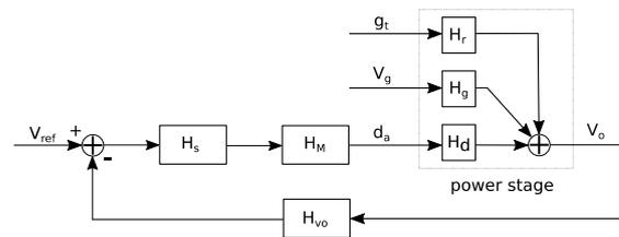
Fig. 1. Small signal equivalent circuit model of Buck converter with voltage control mode.
