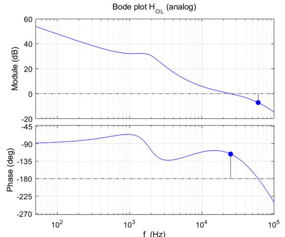
Fig. 2. Bode plot of the analog prototype  $H_{OL}$ .
