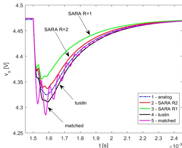
Fig. 7. Voltage  $v_o$  change under the influence of voltage  $v_g$  step change for different transformation methods from domain  $s$  to domain  $z$
