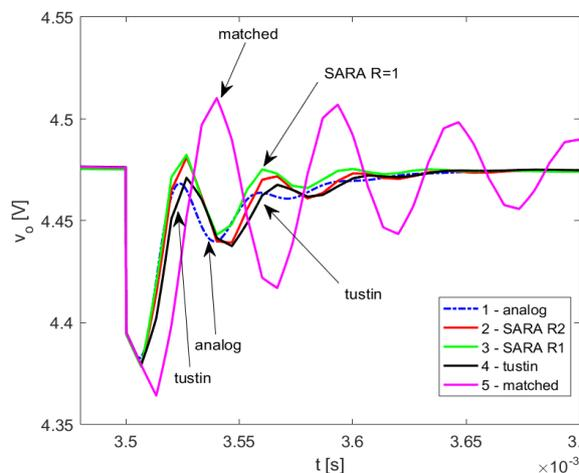
Fig. 8. Voltage  $v_o$  change under the influence of voltage  $g_t$  step change for different transformation methods from domain  $s$  to domain  $z$
