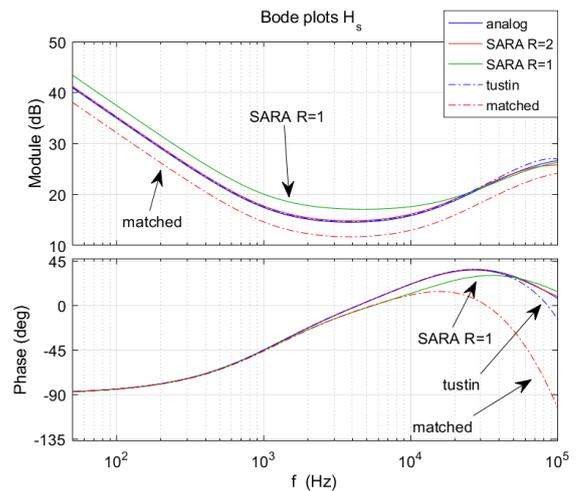
Fig. 3. Bode plot of the transfer function  $H_s$  of control system.
