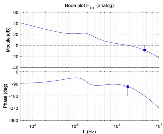
Fig. 6. Bode plot of the analog prototype  $H_{OL}$  with reduced sample rate.
